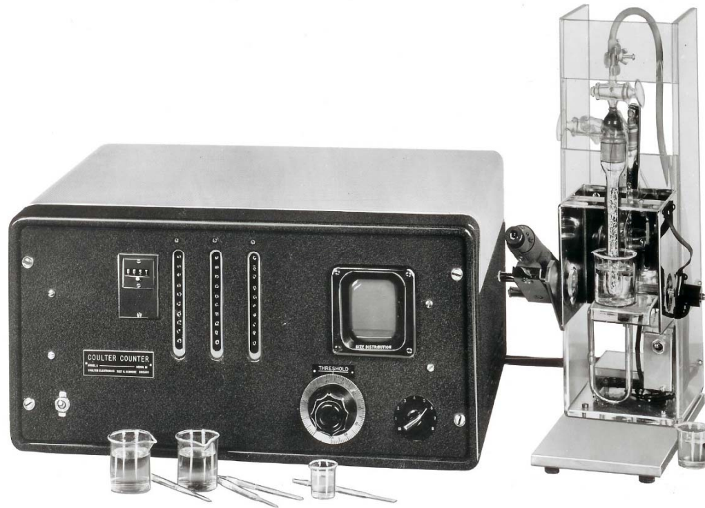
Figure 5.2. An early production Coulter Counter® Model A. 193 According to the panel label, the electronics unit was Coulter Counter, “Model A ---- serial 111,” from “Coulter Electronics...5227 North Kenmore...Chicago.” Production instruments retained the same panel layout as the prototype, but were repackaged to improve presentation (see Figure 4.8), their electronics were less noisy, and their volume-control manometer drew count volumes of better accuracy from the sample beaker on the sample stand’s platform.
