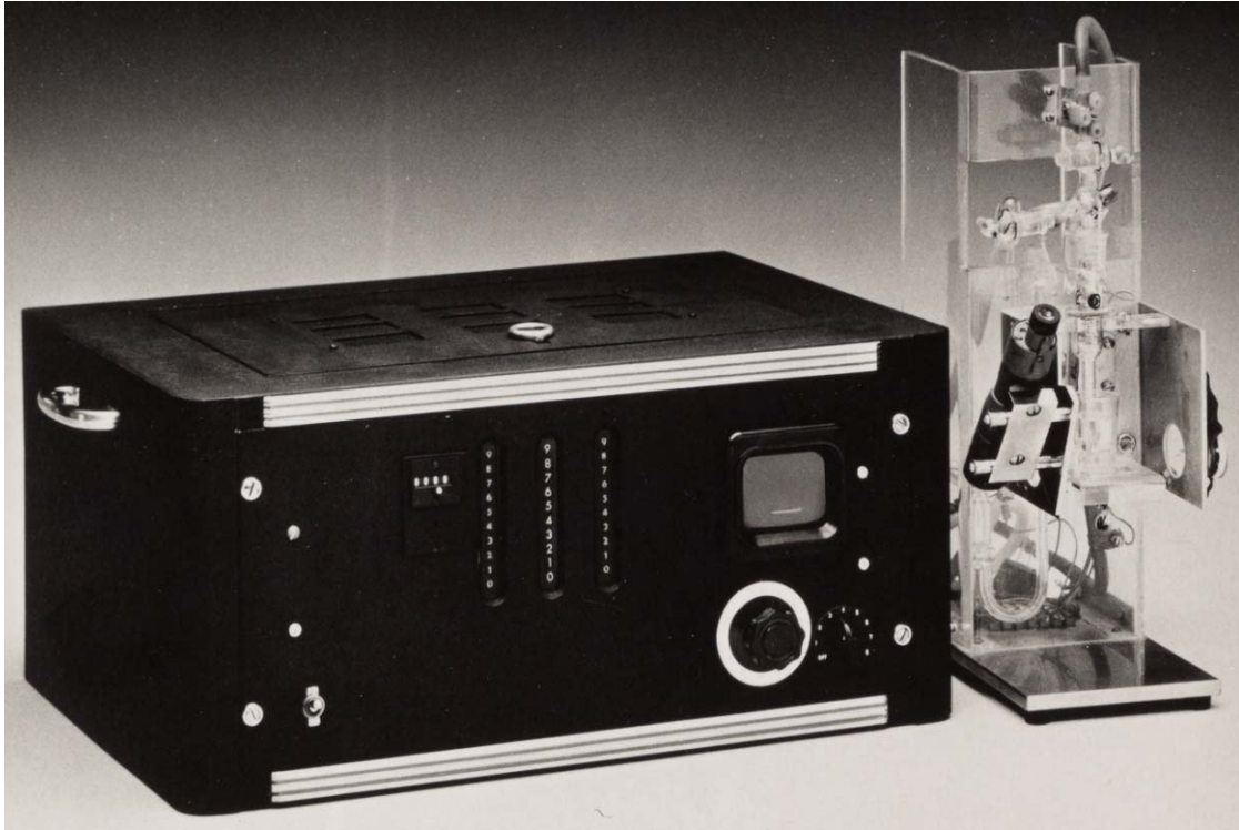
Figure 4.5. ONR laboratory model cell counter. This experimental instrument included refinements gained via work with the integrated instrument (Figure A11.3); WHC Papers.
